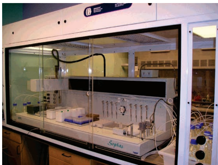
Figure 1. Solvent screening matrix dispensed using Zinsser SOPHAS.
